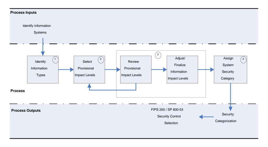
Figure 2: SP 800-60 Security Categorization Process Execution
